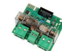
AX LUX ADI module for the management of lights, traffic light or electrobrake Code 16Y007 p. X
